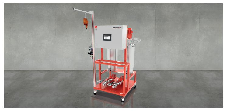
The compomix FI has been specially designed for the impregnation of fibre rovings in vacuum infusion, resin transfer moulding (RTM), pultrusion, and filament winding processes. It ensures the precise metering and mixing of two-component material used for glass, aramid or carbon fibre impregnation (FI). Depending on the application specifics, the compomix FI can be used to either fill a resin bath and
