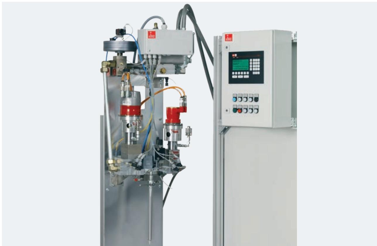
2K-modis is used to handle two component materials. Due to its compatibility and modularity, two modis single component systems can be connected by simply using a mixing block onto the outlet of which a plastic mixer is mounted. Just a suitable material supply and metering unit is required.
