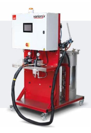
The variomix is a pneumatic driven piston pump type metering and mixing system, used to handle low to high viscosity multi component media such as epoxy resins, polyurethanes or silicones. They can be unfilled, filled as well as abrasive. The
