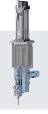
The vectodis metering system is suitable for processing single-component media. The material is discharged in shot or bead form. The material is taken from the original container via a feed pump and fed to a piston metering unit with a servo motor. A material pressure regulator keeps the input pressure at the piston metering unit constant.
